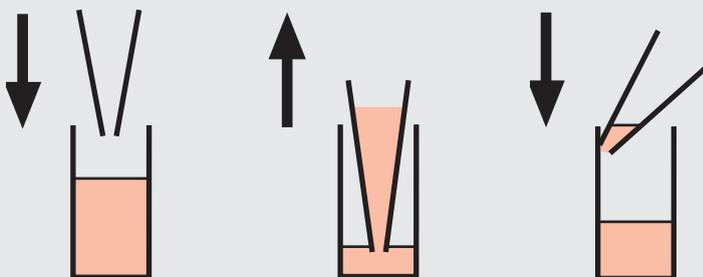
1. Press down button to second stop. Immerse tip a few millimetres into liquid.
