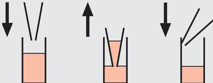
1. Press down button to first stop. Immerse tip a few millimetres into liquid.
